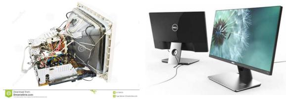
Early Monitors used Cathode Ray Tubes. It was about 30 years ago that these weighty monitors began to be replaced by flat screen technology such as the LCD and LED displays. The Monitor Definition Files used with RISC OS hardware such as the RiscPC were designed for CRT monitors. Monitor Definition Files used with flat screens are much easier to create.
