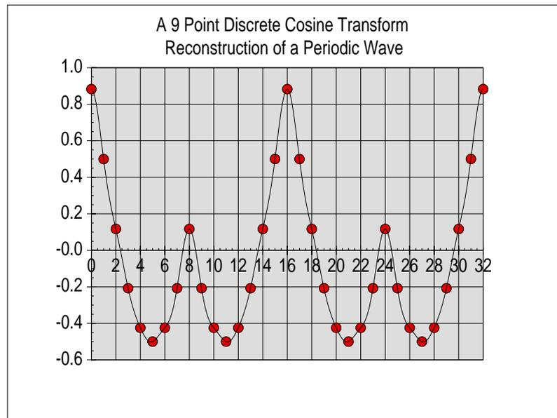
What I would like you to notice is that, outside these original 9 points (numbered 0 to 8), the graph for the points 8 to 16 does not repeat in an identical way. The graph for the points 8 to 16 are a mirror image reflected in the vertical line,  $x = 8$ . Similarly, for points 16 to 32, the graph is a mirror image of the graph for the points 0 to 16 reflected in the line  $x = 16$ .
