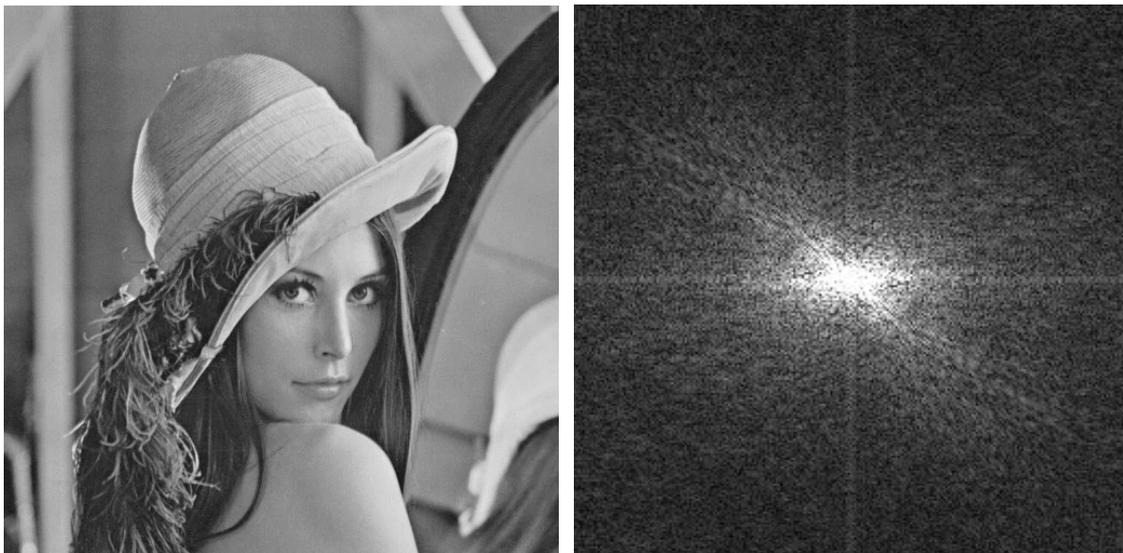
The graphic which looks a little like a galaxy of stars, is a pictorial representation of the Discrete Cosine Transform of this picture of Lenna. The brightness of the 'stars' represents the amplitude of different frequencies with the lower frequencies being near the centre.
