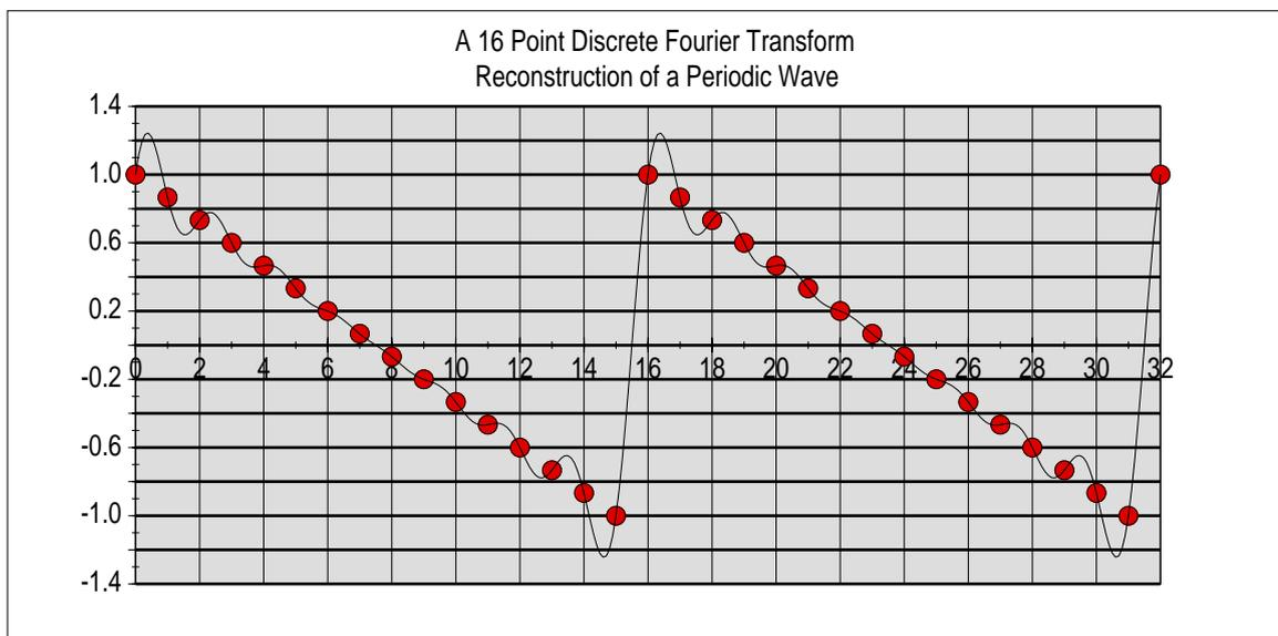
The graphic above shows two cycles of such a reconstructed wave. You will see that the curve which passes through the original 16 points, 0 to 15, is repeated exactly for the 16 points numbered 16 to 31. The graph is repeated exactly every cycle.
