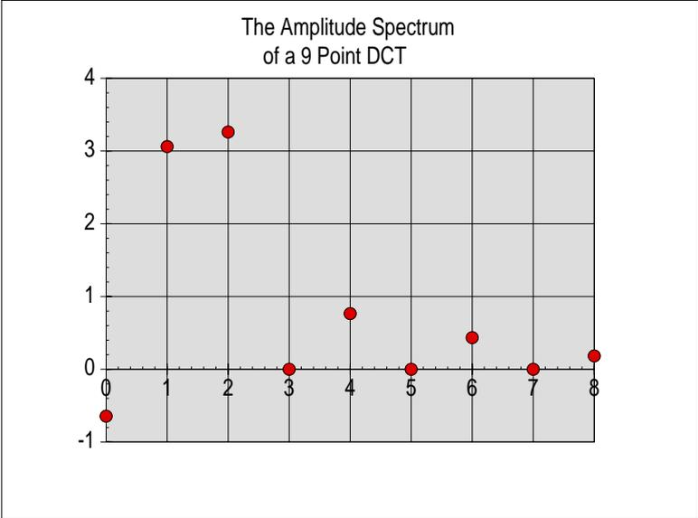
The amplitude spectrum of the 9 point DCT is shown in the above screenshot. The amplitude of the lower frequencies is greater than the amplitude of the higher frequencies. This is typical of DCTs, including multi dimensional DCTs, but is more unusual for a DFT; it is this fact which makes the DCT a more efficient means of compression than the DFT.
